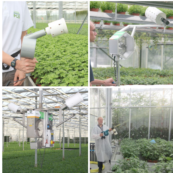
Figure 18: Blowing devices Koppert and Biobest. Left top: Mini-Airbug. Right top: Airbug. Left bottom: Airobug. Right bottom: Nutrigun.
