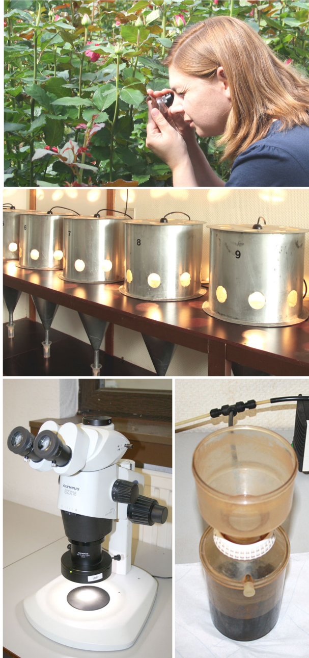
Figure 2: Detection methods. Top: Scouting with a magnifying glass. Middle: Berlese funnel. Left bottom: Microscope. Right bottom: Filtering system.
